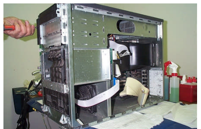
On-site Dismantling & Cleaning of Server in mobile antistatic Workshop
