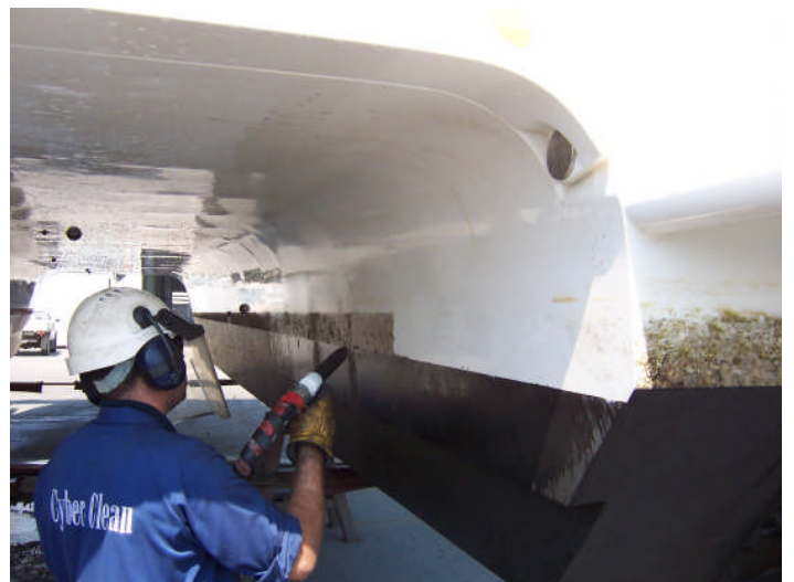
Barnacle Removal without use of water and total protection of hull
